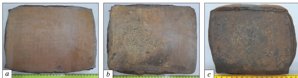
Fig. 10. General view of rolled bilayer plates from (a) Ti64, and (b) LCB sides, and (c) 4-layers plate from Ti5553 side
