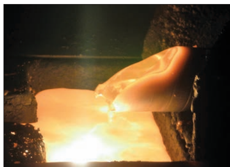
Fig. 3. Process of melting a layer of multilayered ingot
