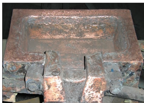
Fig. 2. Copper water-cooled mould
