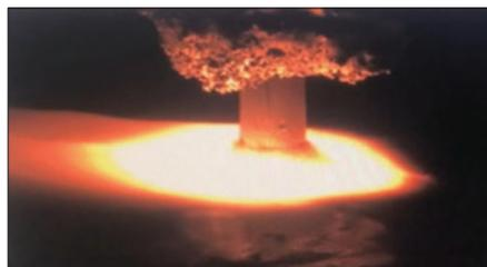
*Fig. 11.* xBeam process configuration with melting the cored wire feedstock by energy accumulated in the melt pool
