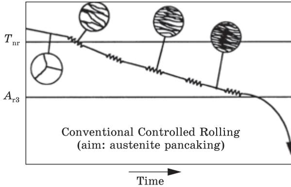
*Fig. 3. Schematic time-temperature diagram of conventional controlled rolling, showing the deformed microstructure between passes*
