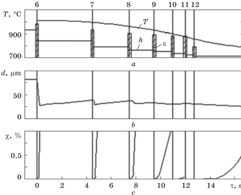
*Fig. 10.* Temperature and deformation mode of rolling (*a*), change in (*b*) and kinetics of austenite recrystallization in the finishing group of stands (*c*);  $T$  — rolling temperature;  $h$  — rolling thickness;  $\varepsilon$  — relative compression [42]
