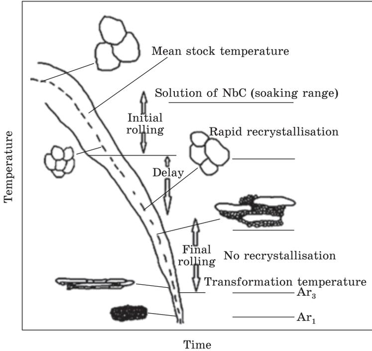
*Fig. 6.* Schematic representation of various processes occurring during control rolling of C-Mn-Nb steels [34]
