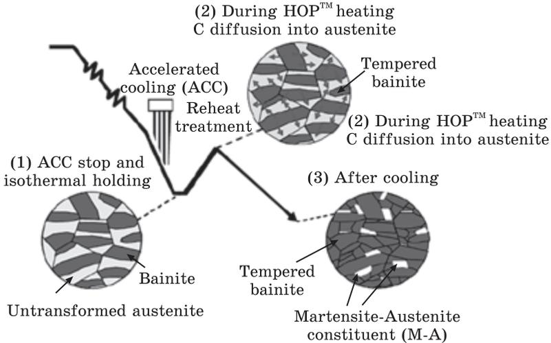
*Fig. 7. Microstructure control by induction heating technology [36] (HOP indicates the heat treatment on-line process)*
