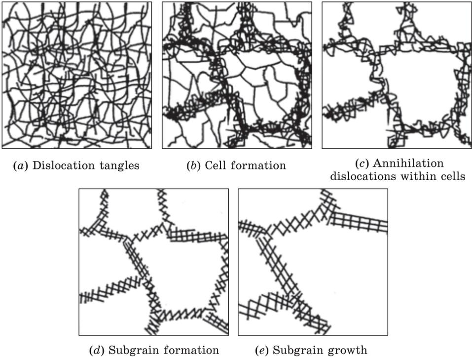
*Fig. 9.* The stages of recovery with the first cells formed due to the rearrangement of dislocations; then, subgrains are formed and grow due to annihilation of dislocations [38]
