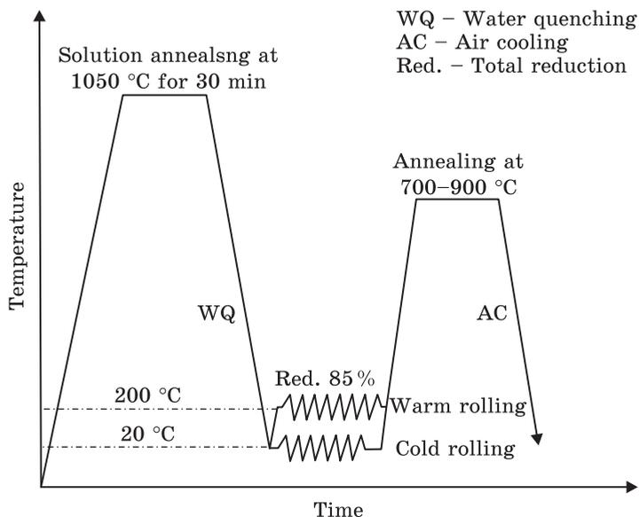
Fig. 8. Scheme of advanced thermomechanical processing [37]
