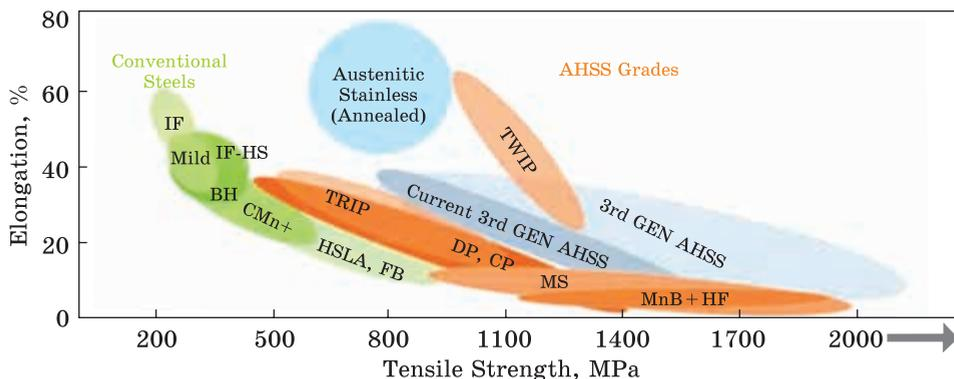
Fig. 1. Graphic representation of the classification of modern types of steel for cold forming [18]
