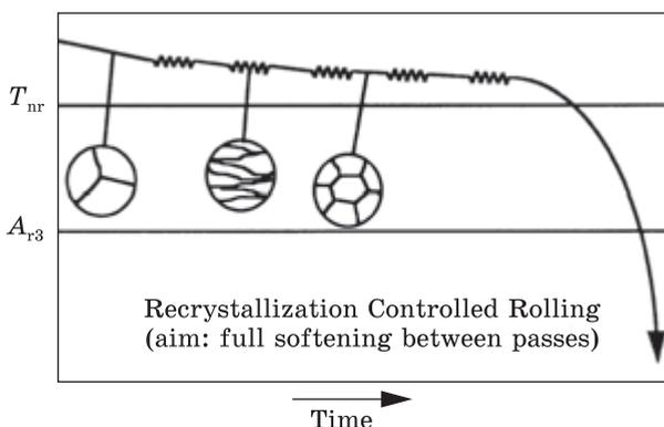
Fig. 2. Schematic time-temperature diagram of recrystallization controlled rolling showing the recrystallized microstructure between passes.  $T_{nr}$  ( $A_{r3}$ ) — the no-recrystallization (phase transformation) temperature [20]
