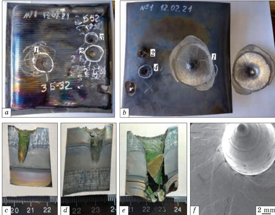
*Fig. 16. Triple Ti-6Al-4V/CP-Ti/T110 plate after ballistic tests [29]: general view from Ti-6Al-4V alloy side (a) and from T110 alloy side showing delaminated fractured area near B-32 (12.7 mm) projectile crater (b); cross sections of the plate near penetration channels of B-32 (7.62 mm) projectiles from Ti-6Al-4V alloy side (c) and T110 side (d) as well as 12.7 mm calibre from Ti-6Al-4V alloy side (e); delaminated back T110 surface near 12.7 mm bullet core stuck (f)*
