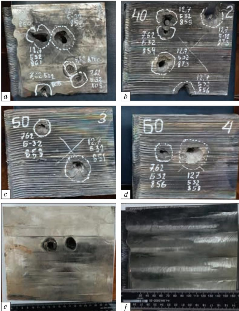
Fig. 9. Front view of Ti-6Al-4V plates of different thickness (*a* — 30 mm, *b* — 40 mm, *c* — 50 mm, *d* — 60 mm) after ballistic tests. Backsides of 30 mm plate pierced with 12.7 mm projectiles (*e*) and not pierced 50 mm plate (*f*) are also shown
