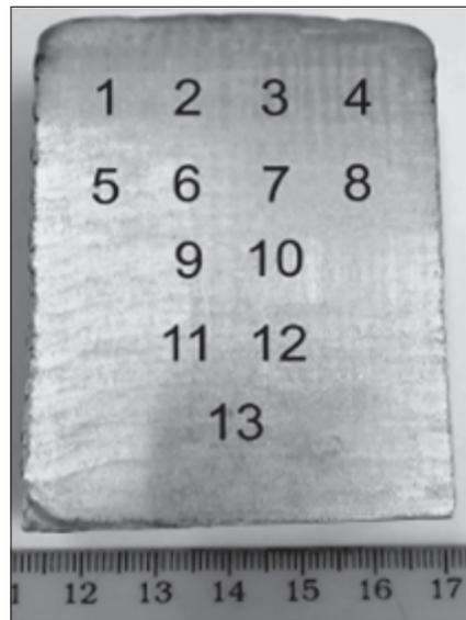
Fig. 30. Areas of the printed samples used to the hardness measurements [50]
