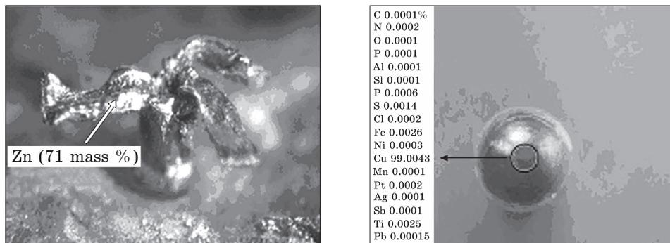
Fig. 9. Copper target after the experiment with traces of solidified silver-white 'lava' on its petals, poured out from the centre of the exploded target [27]
