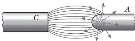
Fig. 7. Sketch of self-focusing of the electron beam on the concentrating anode surface, which excites a soliton-like density pulse in its near-surface layer, converging to the symmetry axis [27]
