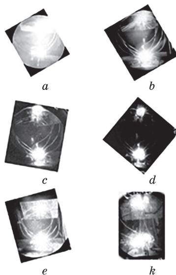
space. Then, the glow becomes less bright. The next frame shows a spherical glow (Fig. 6, b). During the next 3–4 ms, no dynamics is observed (Fig. 6, b, c, d). Then the luminous ball begins to crumble into many small ‘balls’. In a series of experiments, it was noticed that the ‘ball’ first rises by 15–30 cm above the surface of the dielectric cover, and then crumbles (Fig. 6, f).
