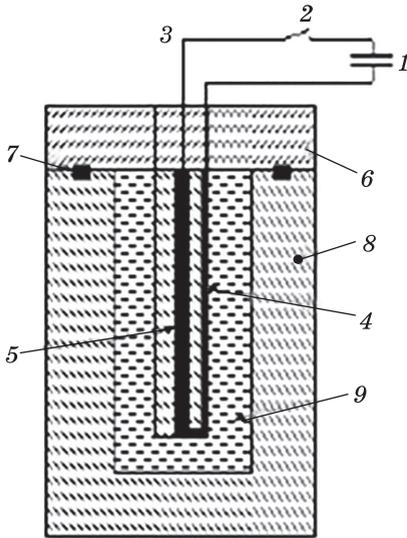
Fig. 5. Scheme of the experiment: 1 — capacitor bank, 2 — arrester, 3 — cable, 4 — foil, 5 — electrode, 6 — polyethylene cover, 7 — seal, 8 — explosion chamber, 9 — distilled water [25]
