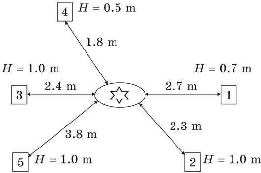
Fig. 3. Scheme of location of detectors during the explosion of conductors [22]
