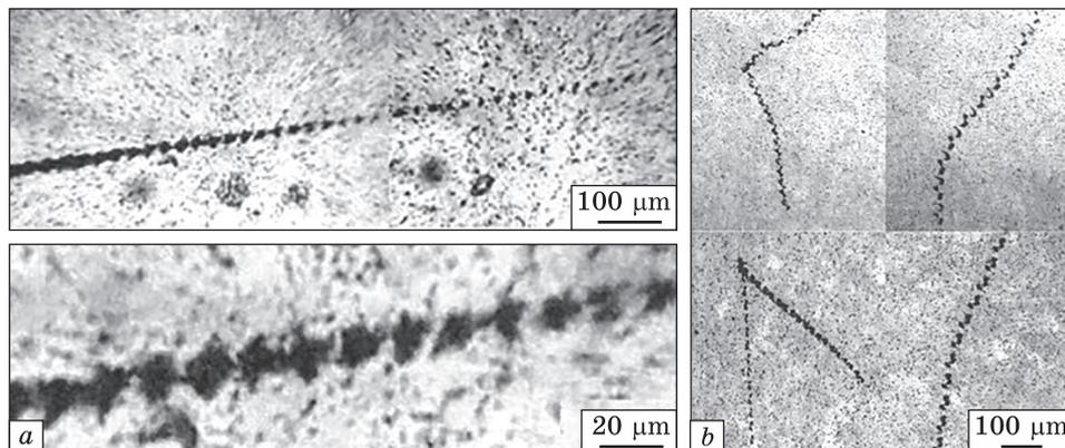
Fig. 4. Micrograph of traces registered during (a) the test of the surge suppressor and (b) electric explosion of wires [22]
